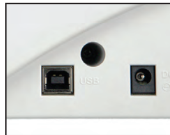
USB port automates plug and play installation.
